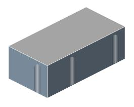
Three piece slab system with 2MM micro-chamfer and 2MM hidden spacer lugs on 75MM center-to-center spacing.
