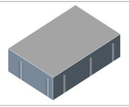
Flat top, single piece paver system with 2MM microchamfer and 2MM hidden spacer lugs on 75MM center-to-center spacing.
